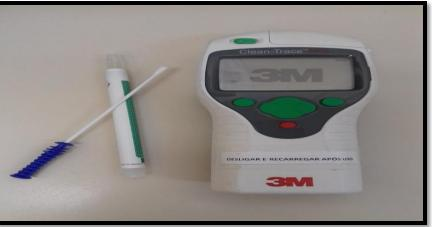
Special apparatus for measuring vibration in Ultrasonic cleaner • Luminometer: ATP test for cleaning monitoring purposes
